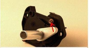
to aid in reassembly, preposition servo using repair part as a tool, so the stop arm covers this screw.
