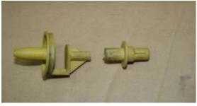
The shaft that connects the stepper motor to the blend door fails as shown above.
